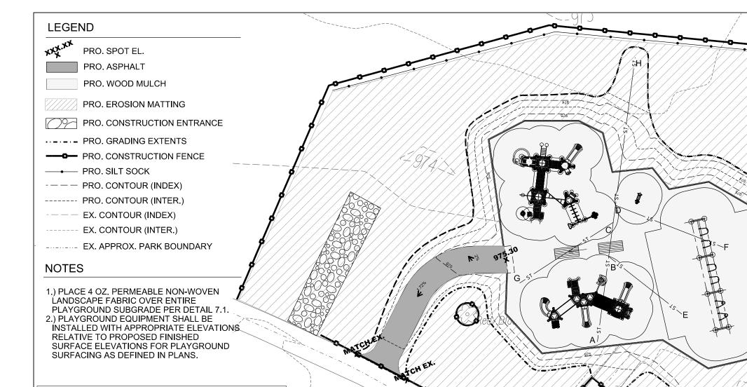
EDGE OF PLAYGROUND BORDER TIMBERS: 975.47 ELEVATION OF FINISHED PLAYGROUND SURFACE: 975.30 PLAYGROUND SUBGRADE ELEVATION: 974.30 ASPHALT AT PLAYGROUND ELEVATION: 975.30
